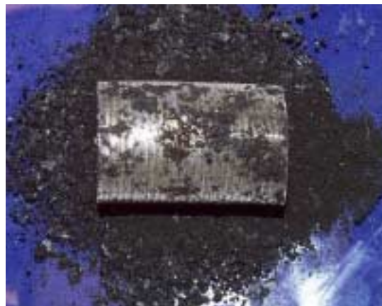
Figure 1: Copper Scale collected from a Solar Plant
