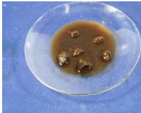
F4: Seriously damaged fluid, residues non-redissolvable
