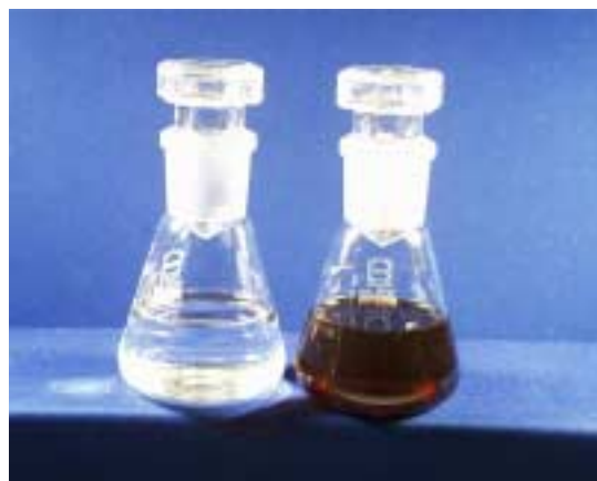
Figure 2: Un-used Solar Fluid (left, pH 8.2), compared to overheated Fluid (pH 6.8)
